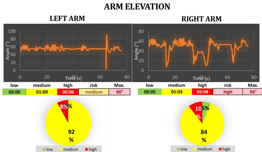
Figure 25. ScaleFit analysis of the arm elevation of the participant 3 from IPS-IMMA.
