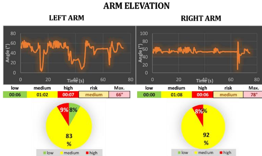
Figure 26. ScaleFit analysis of the arm elevation of the participant 10 from IPS-IMMA.
