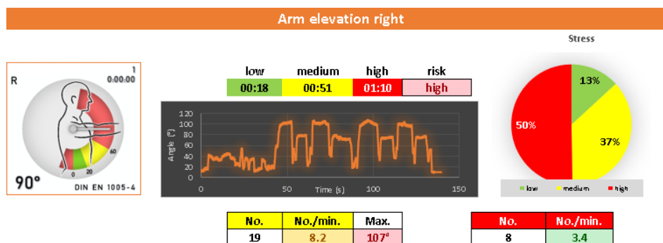
Figure 60. Right arm elevation of Participant 3 (Exoskeleton record).
